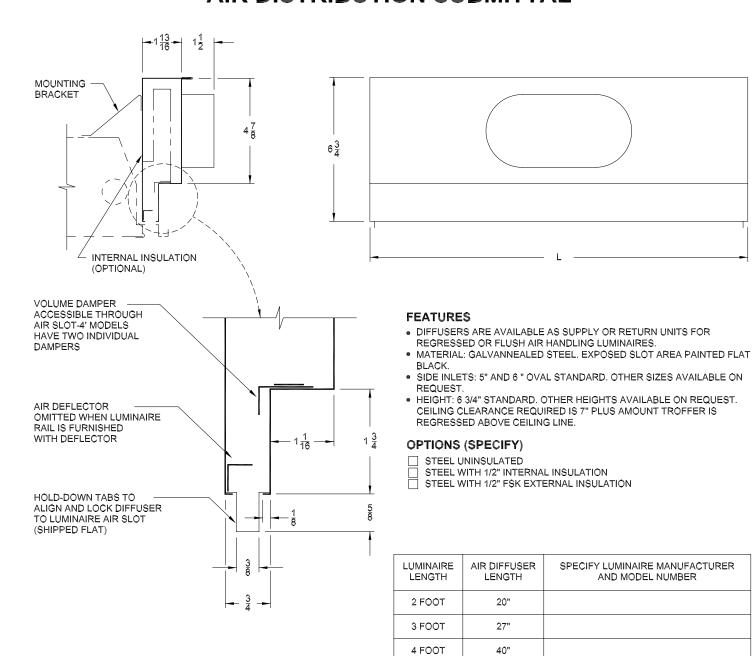
DETAIL COORDINATION DRAWING OF TROFFER DIFFUSER AND SPECIFIC JOB LUMINAIRE AVAILABLE FROM FACTORY ON REQUEST.
